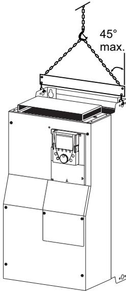
ALTIVAR 71 drives up to ratings ATV71HD15M3X and ATV71HD18N4 can be removed from their packaging and installed without a handling device.
