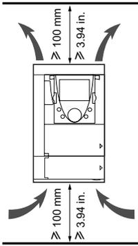
Install the drive vertically at  $\pm 10^\circ$ .
