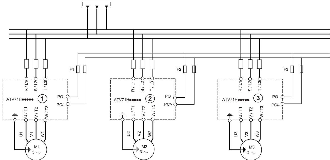
Drives ①, ② and ③ must not be more than one size apart when they are connected in this way.
