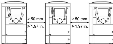
**Type B mounting** Drives mounted side by side, with the protective cover removed (the degree of protection becomes IP20)
