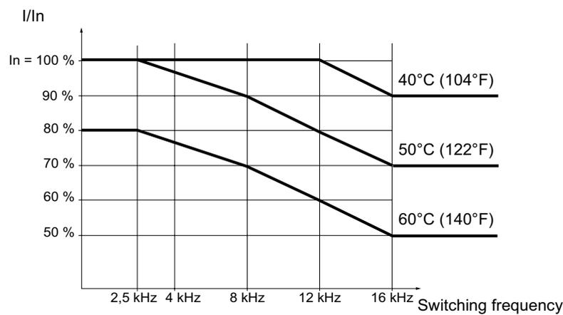
For intermediate temperatures (e.g. 55°C [131°F]), interpolate between 2 curves.
